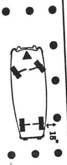
STEP 5 Continue backing into proper position, leaving wheels turned out.
